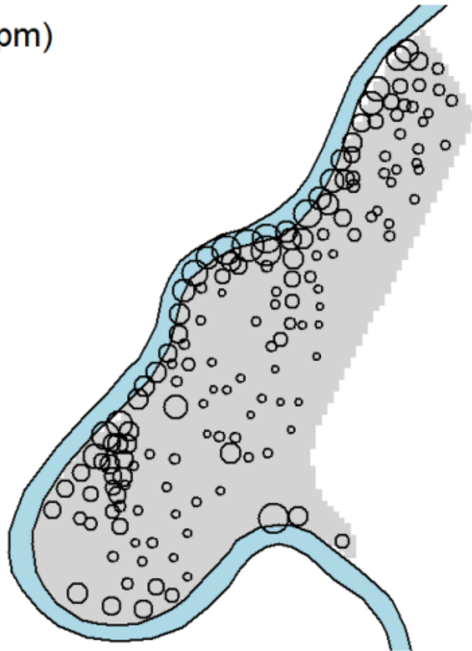
Figure 61. Plot of zinc concentrations in soil near River Meuse, The Netherlands.
