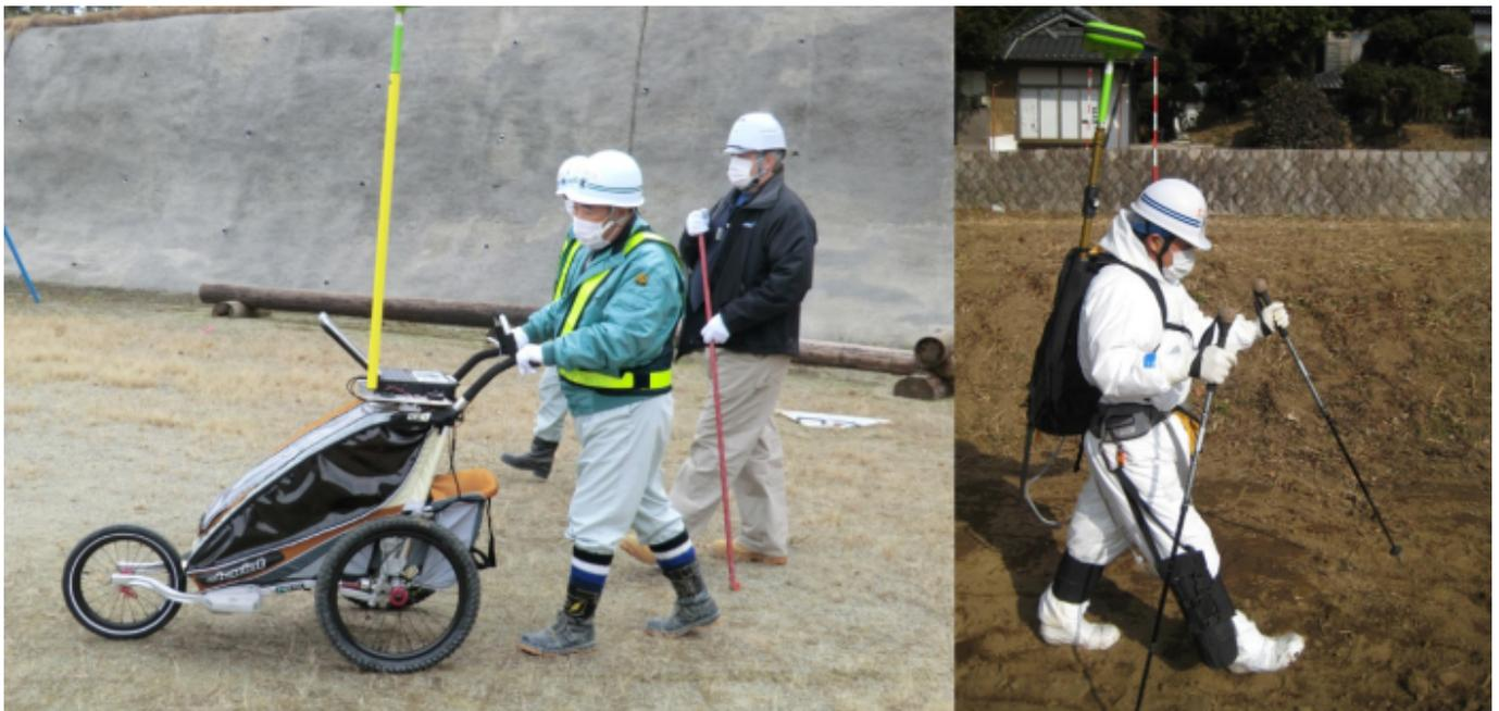
**Figure 103. ScanPlot<sup>SM</sup> “buggy” (left) and back-pack deployment (right).**
