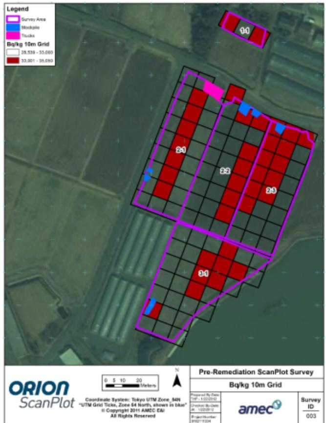
Figure 105. Left: Average combined cesium-134 and 137 levels created using the Zonal Statistics tool set. Right: Identification of 10-meter grid cells (red) with levels exceeding risk-based thresholds (red).
