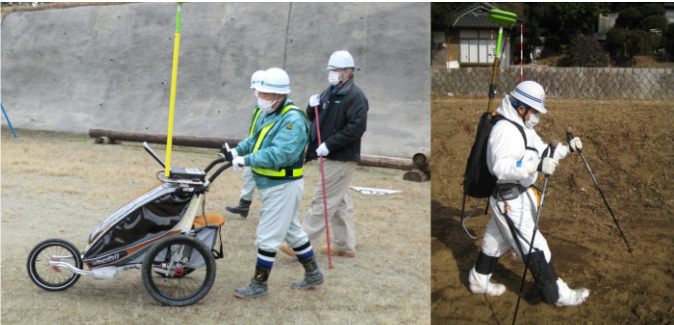
Figure 103. ScanPlot SM “buggy” (left) and back-pack deployment (right).
